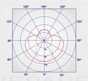
photometric curves of Transparent 1x36 luminaire
